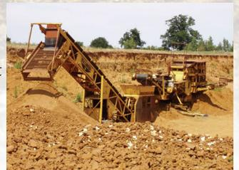
Mill Drove Quarry at Middleton, extracting Carstone for hardcore and building material.
